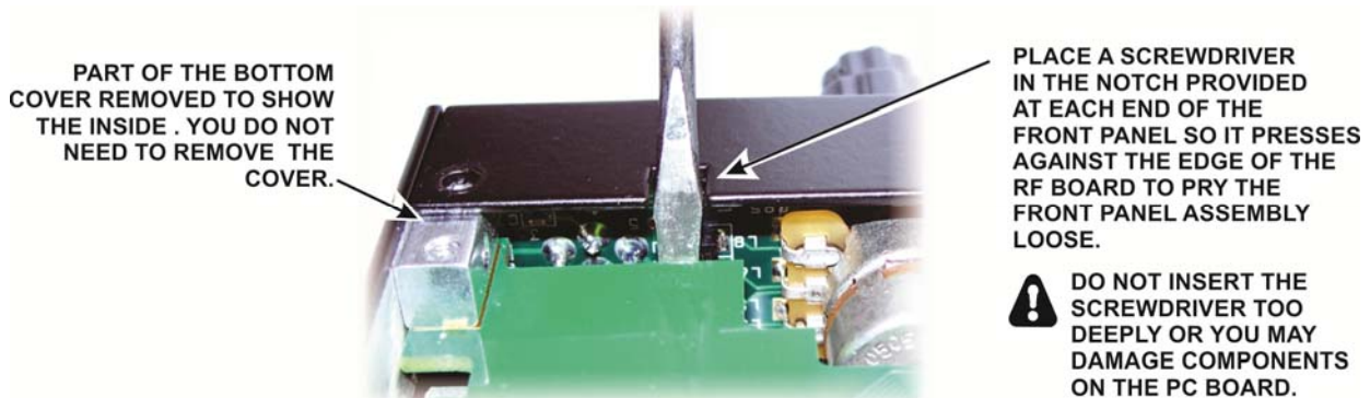
Figure 5. Disengaging the Front Panel Assembly.
